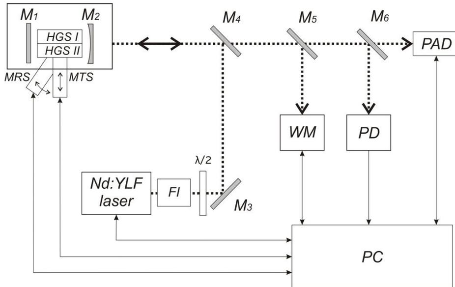
Figure 2. Experimental setup: Nd:YLF laser – pump laser, FI – Faraday isolator;  $\lambda/2$  – half-wave plate;  $M_1$ - $M_6$  – mirrors; MTS – motorized translation stage; MRS – motorized rotation stage; WM – wavelength meter; PD – pyroelectric photodetector; PAD – photo-acoustic detector; PC – computer
